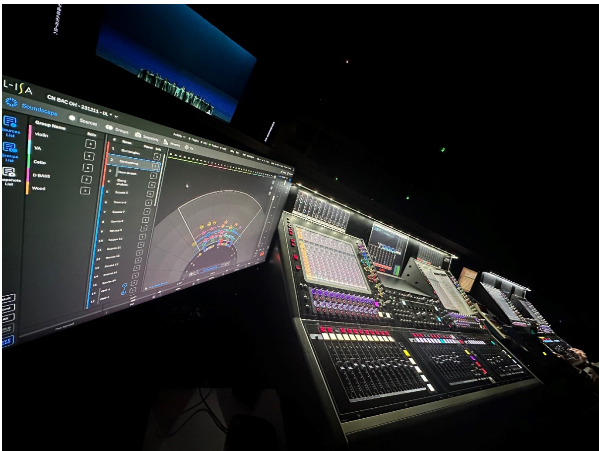
Redundancy in live audio: Two DiGiCo Quantum 5 consoles mirrored at the FOH position of the opera 'The Canal Ballad' at the opening performance of the Beijing Performing Arts Centre in December 2023. (Image courtesy of Racpro)
